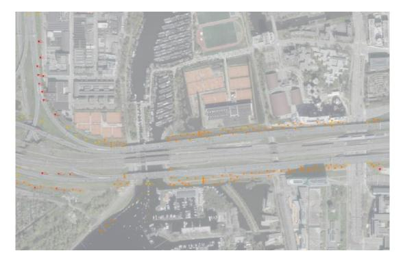
The various colours of the soil survey sites correspond to the various depths, ranging from 15 to 35 metres.
